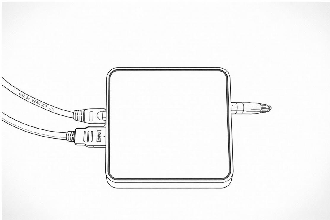
2. Press and hold the front power button of the CT1820, then connect the power cable.
